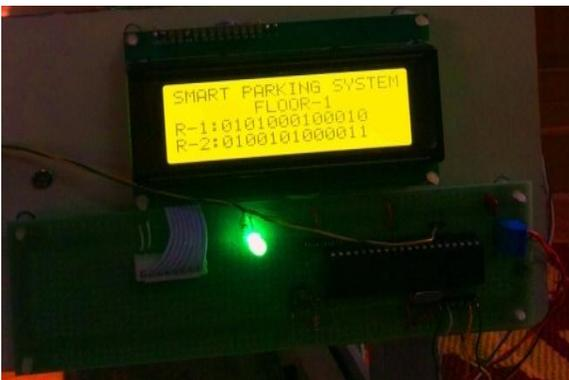
**Fig-8:** Show the status of parking slots on 1<sup>st</sup> floor LCD Display
