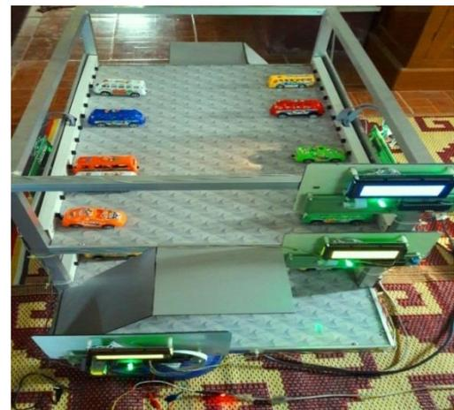
**Fig-11:** Prototype of smart parking system
