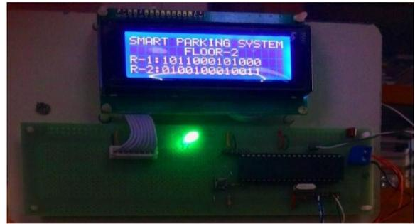
**Fig-9:** Show the status of parking slots in 2<sup>nd</sup> floor LCD Display
