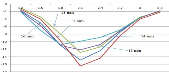
**Fig.3 Return loss function with different ground plane lengths**
