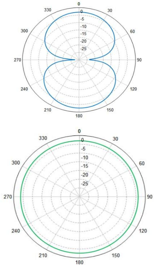
**Fig.8** (a) E-plane and (b) H-plane radiation pattern at 1.83 GHz
