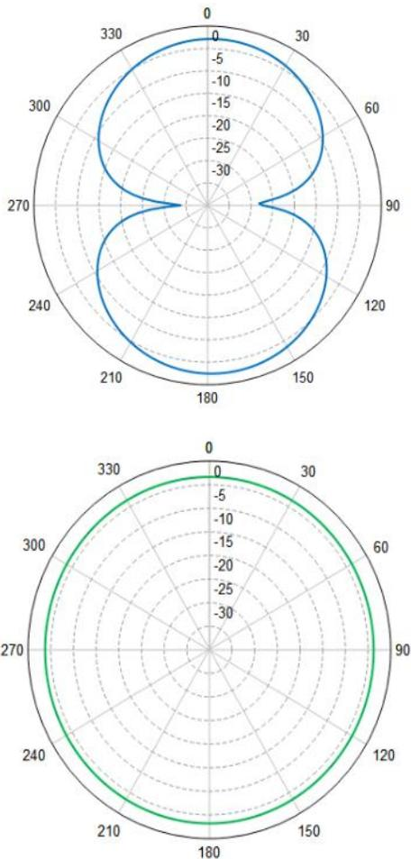
**Fig.7** (a) E-plane and (b) H-plane radiation pattern at 2.1 GHz
