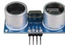
Figure.7. Ultrasonic ranging module HCSR-04
