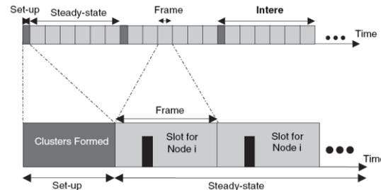
Figure 2: Time line showing LEACH operation
