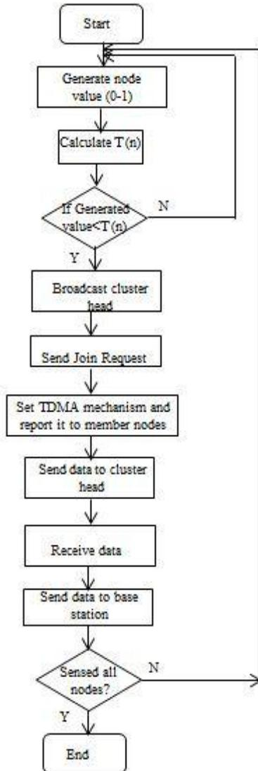
Figure 3: The work process of LEACH protocol
