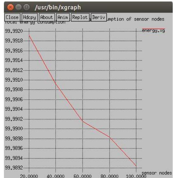
Figure 7: Total energy consumption of sensor nodes
