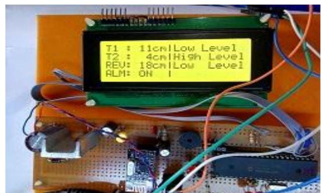
Figure 11. The water level of Tank2 is reached high level (4cm)
