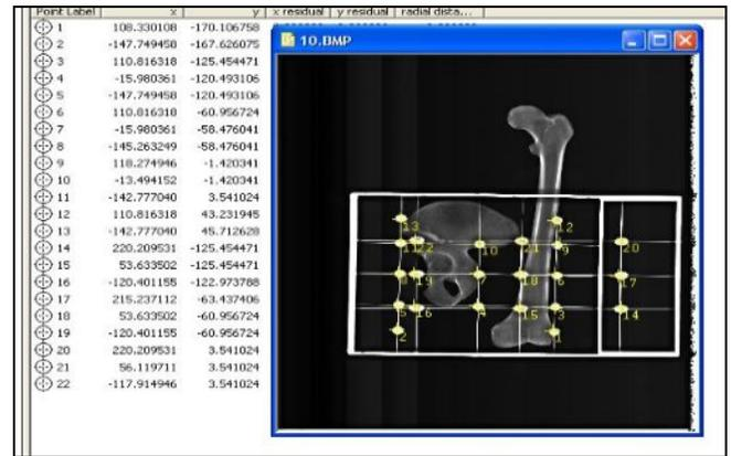
Figure 8 Labeled target points for Statscan small metal frame image taken at 10 degrees.
