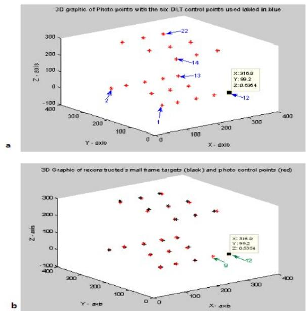
Figure 9 Labeled control points used in Statscan small frame reconstructed (a), and both control frame points (red) plotted together with respective reconstructed points (black) (b).
