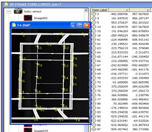
Figure 4 Measured target points of Statscan 14 degree image for the big metal frame.
