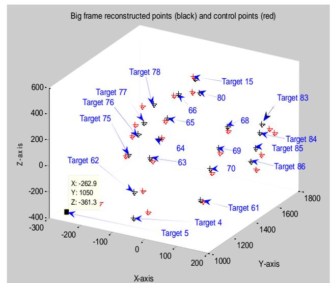
Figure 6 3D graphic of the Statscan big frame reconstructed points (black) and control points (red) using 5 degree and 53 degree image combinations.
