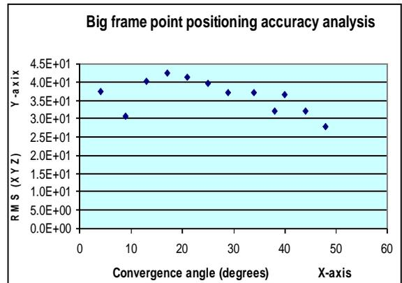
Figure 5 Plot of Statscan big frame image orientations against point positioning accuracy RMS (XYZ).
