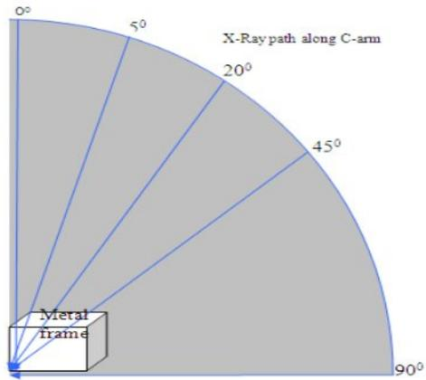
**Figure 3** Schematic of different X-ray scan orientation angles along the Statscan’s C-arm (not scaled).
