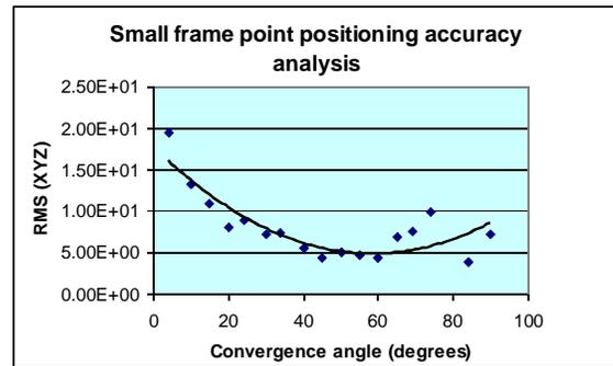
**Figure 11** Positioning accuracy RMS (XYZ) against convergence angle for Statscan small frame (0 – 90 degree images).
