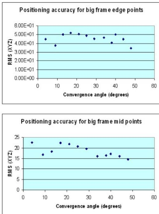
Figure 7 Big frame positioning accuracy for edge points (a) and mid points (b)
