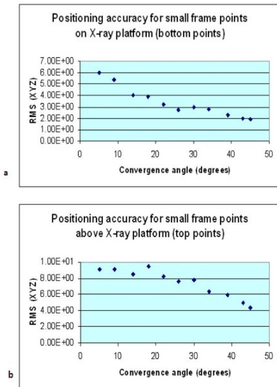
**Figure 10** Positioning accuracy for small frame bottom (a) and top (b) points on the Statscan X-ray platform.
