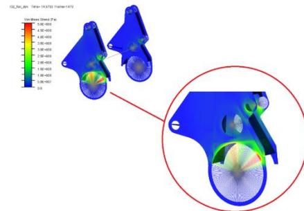
Fig 4. Road with the R32 m radius front axle stress distribution and scale
