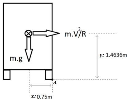
Fig. 3. Analytical vehicle overturn radius calculation
