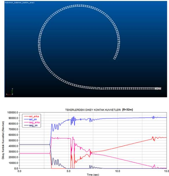
Fig. 2. R32 Road model and wheel vertical contact forces
