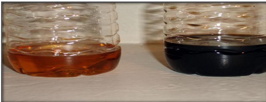
**Fig.1 . Fresh and used oil representation used in concrete**
