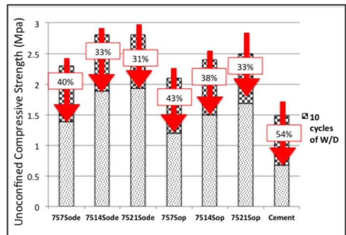
**Figure 3.** Evolution of compressive strength after mouillage-sechage test.
