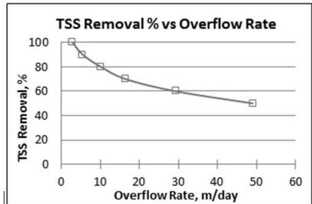
Fig. 7. TSS Removal % vs overflow rate curve.
