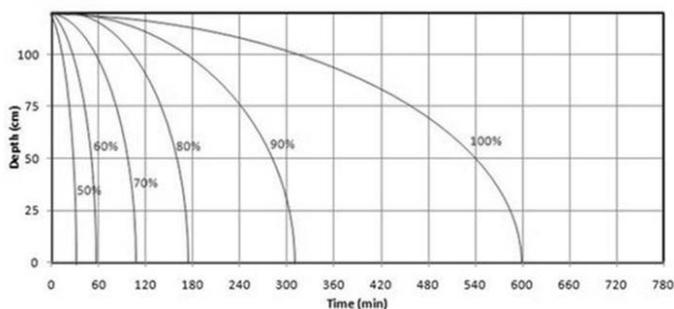
Fig. 5. Iso-removal curves obtained from sedimentation analysis.
