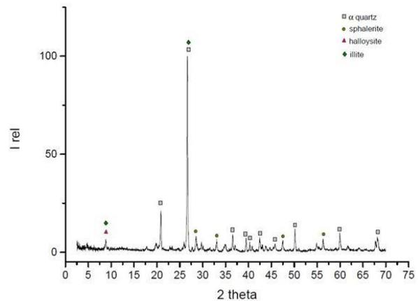
Fig. 11. X-ray diffractogram for the sediment.
