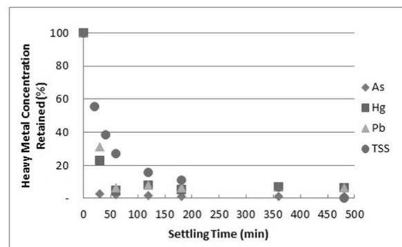
Fig. 8. Heavy metal and TSS concentrations change measured at port 100 cm from the bottom during sedimentation.
