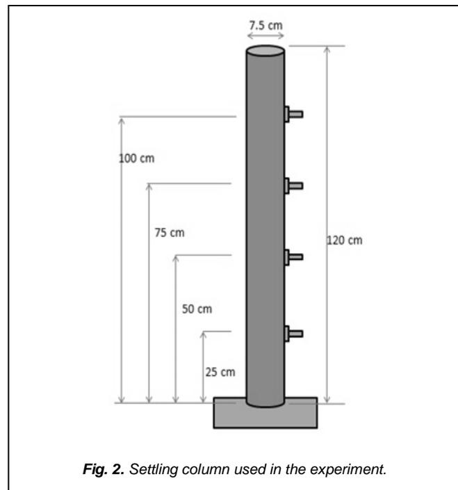
**Fig. 2.** Settling column used in the experiment.
