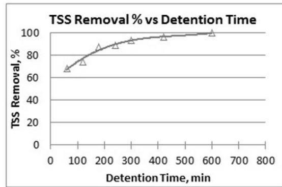
Fig. 6. TSS Removal % vs detention time curve.
