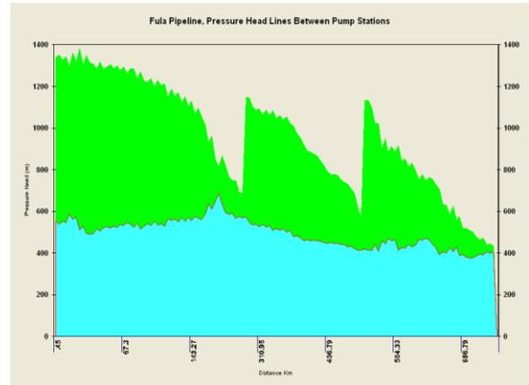
**Fig 8:** Fula pipeline profile and pressure transverse between pump stations (3 PS, throughput=40000 BOPD)
