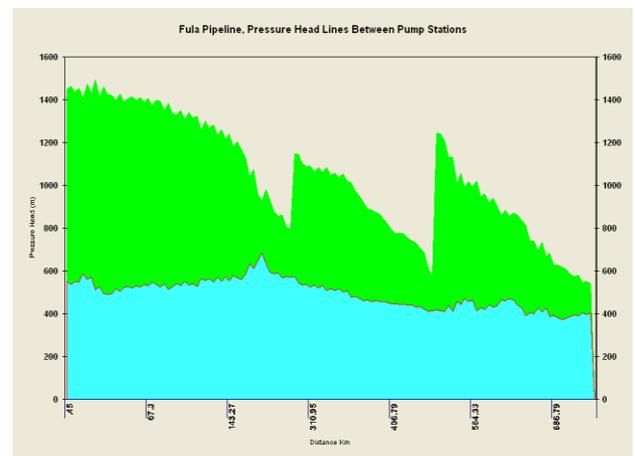
**Fig 8:** Fula pipeline profile and pressure transverse between pump stations (3 PS, throughput=40000 BOPD)
