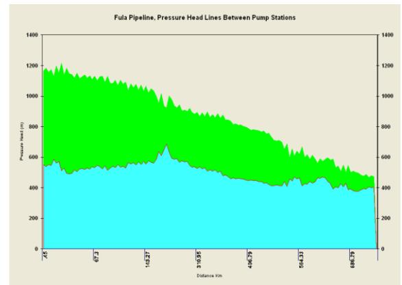
**Fig 5:** Fula pipeline profile and pressure transverse between initial and terminal pump stations (Discharge pressure=5500 kPa, throughput=10000 BOPD)
