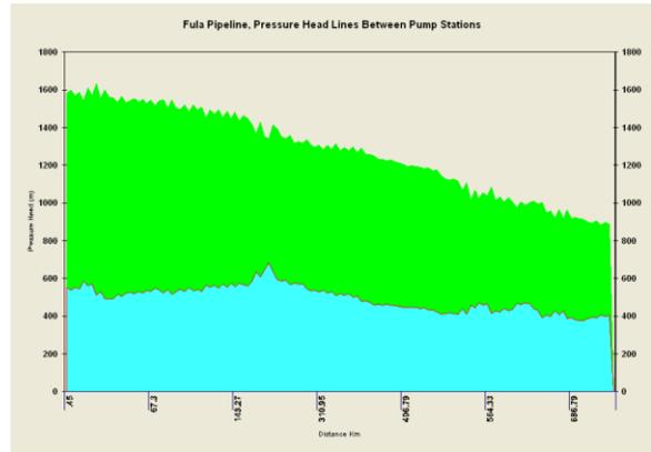
**Fig 4:** Fula pipeline profile and pressure transverse between initial and terminal pump stations (Discharge pressure=9200 kPa, throughput=10000 BOPD)
