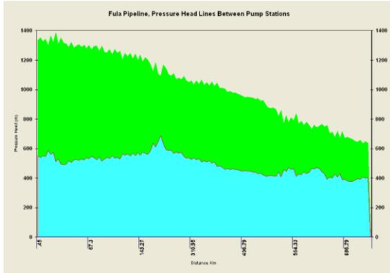
**Fig 6:** Fula pipeline profile and pressure transverse between initial and terminal pump stations (Discharge pressure=7000 kPa, throughput=15000 BOPD)
