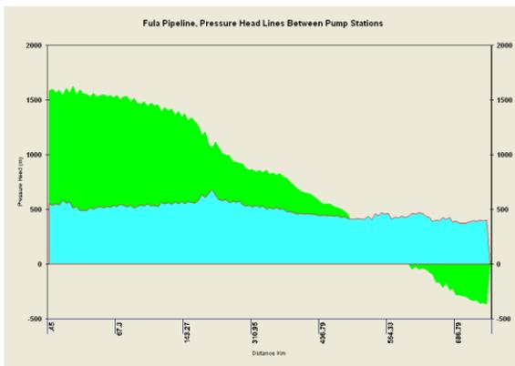
**Fig 7:** Fula pipeline profile and pressure transverse between initial and terminal pump stations (Discharge pressure=9200 kPa, throughput=40000 BOPD)
