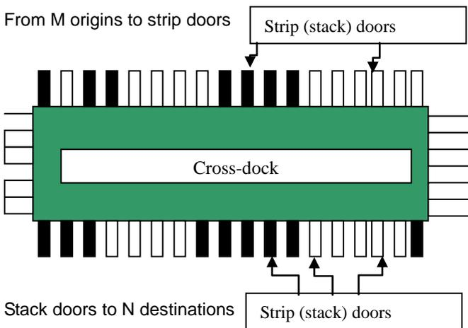
**Fig. 1** Schematic picture of a cross-dock
