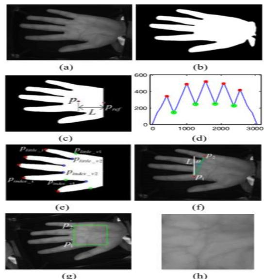
Fig. 2: Illustrations of palm vein ROI extraction (from (a) to (h)): (a) original hand image, (b) binary hand image, (c) reference point and centroid, (d) RDF, (e) description of five fingertips and four finger valleys, (f) the angle  $\theta$  between line  $p_1 p_2$  and vertical line  $L$ , (g) normalized palm vein image, and (h) palm vein ROI.
