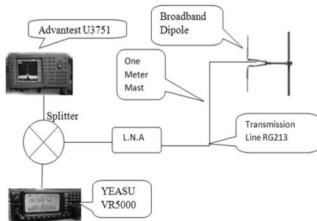
**Figure 2: Testing Equipment Arrangement**
