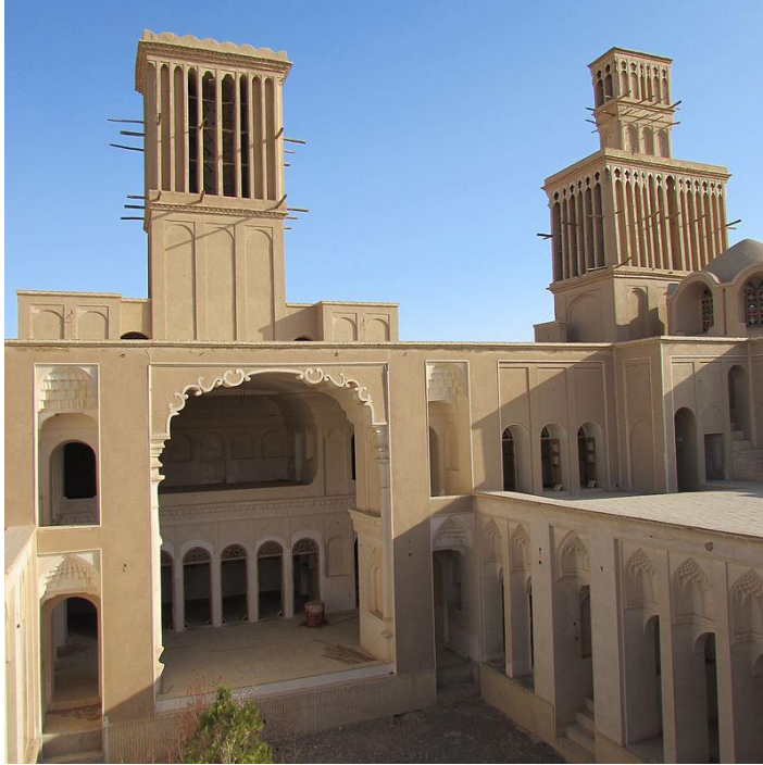
Fig. 4. Wind catchers served as a cooling system (Seyed Aliagha house-Abarkouh)
