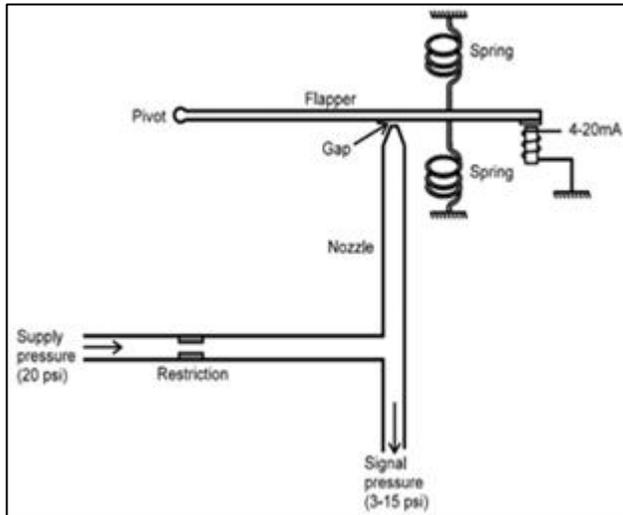
Fig. 6. Current to pressure converter
