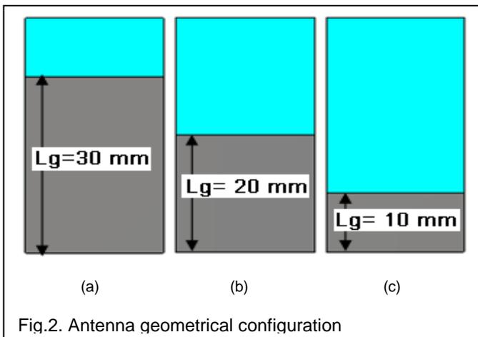
The simulated results in terms of return loss plots for the structures shown in fig.2 with reducing ground plane are shown in fig.3.
