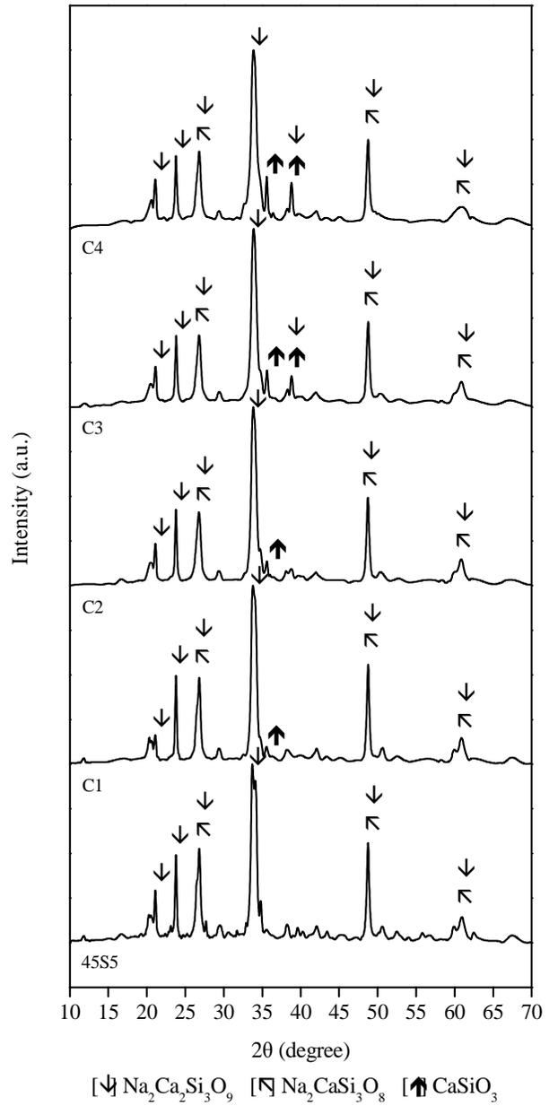
Figure 2: XRD Patterns of Bioactive Glass - ceramics
