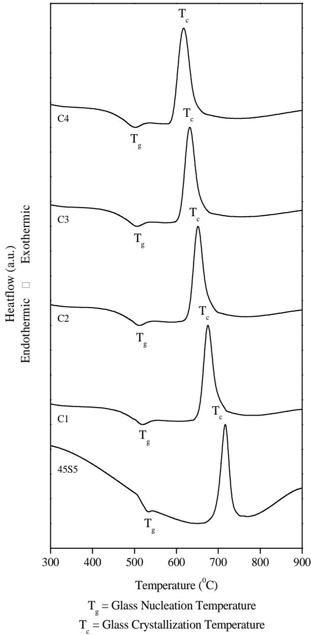
Figure 1: DTA Traces of Bioactive Glasses
