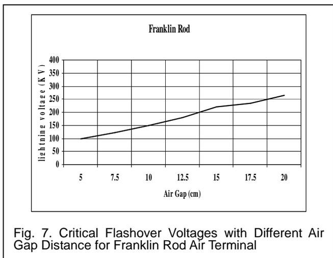
Fig. 7. Critical Flashover Voltages with Different Air Gap Distance for Franklin Rod Air Terminal
