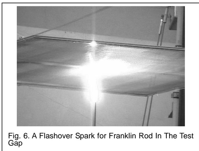
Fig. 6. A Flashover Spark for Franklin Rod In The Test Gap
