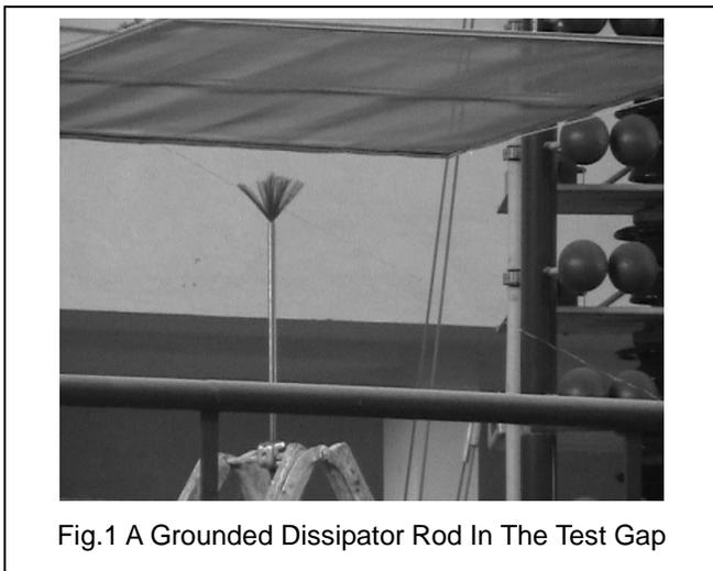
Fig.1 A Grounded Dissipator Rod In The Test Gap
