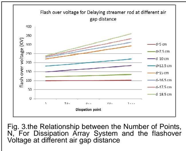
Fig. 3. the Relationship between the Number of Points, N, For Dissipation Array System and the flashover Voltage at different air gap distance
