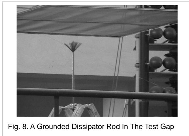
Fig. 8. A Grounded Dissipator Rod In The Test Gap
