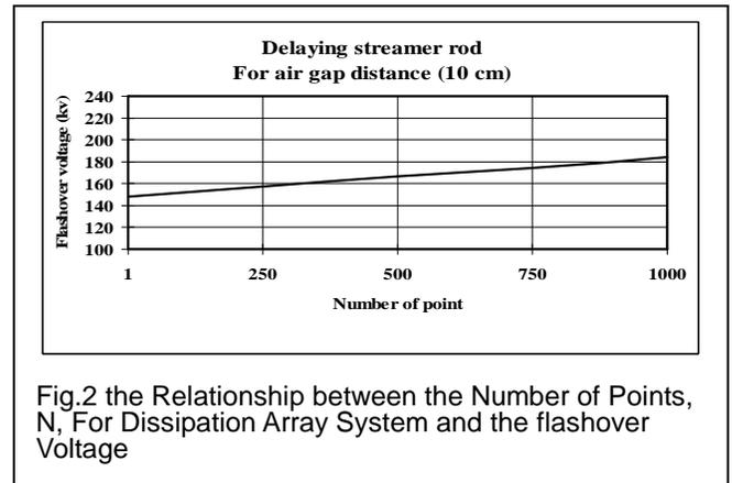
Fig.2 the Relationship between the Number of Points, N, For Dissipation Array System and the flashover Voltage
