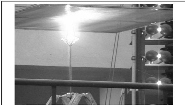
Fig. 9. A Flashover Spark for Delaying Streamer Air Terminal In The Test Gap
