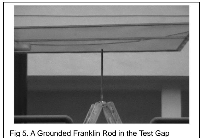
Fig 5. A Grounded Franklin Rod in the Test Gap
