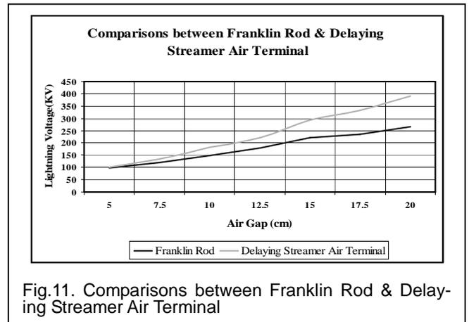
Fig.11. Comparisons between Franklin Rod & Delaying Streamer Air Terminal
