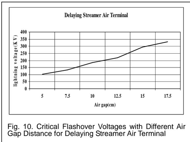
Fig. 10. Critical Flashover Voltages with Different Air Gap Distance for Delaying Streamer Air Terminal
