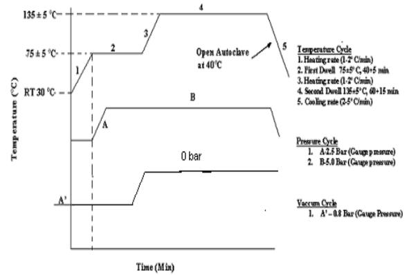
**Fig.15.** Recommended cure cycle for 913 monolithic parts, where the vacuum is cut off gradually after increasing the external pressure.
