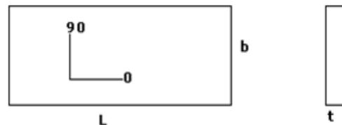
Length L= 20 mm, width b= 10 mm, thickness t= 2 mm.
