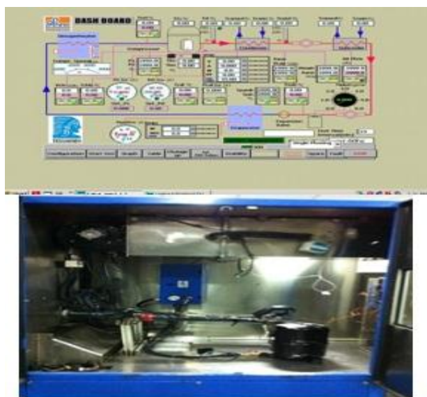
Fig. 5 Dash Board diagram of Calorimeter Test Rig
