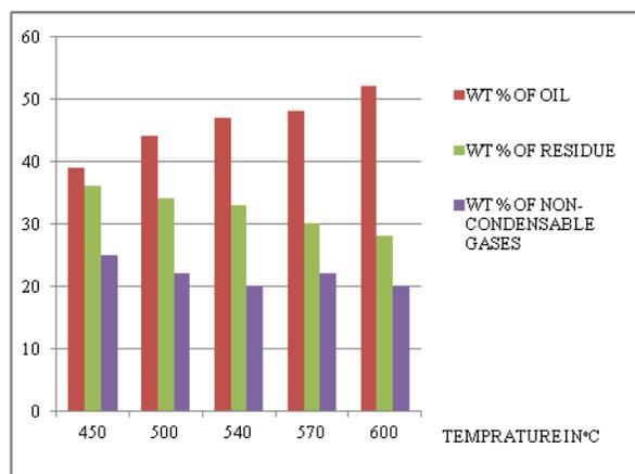
**Fig.2:** Influence of temperature on the yield obtained from mustard de-oiled cake at different temperatures when heated at the rate of 15°C/Min.
