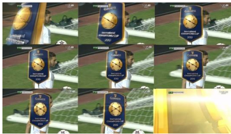
Fig -3: Logo frame transition and sudden increase in brightness in last logo frame
