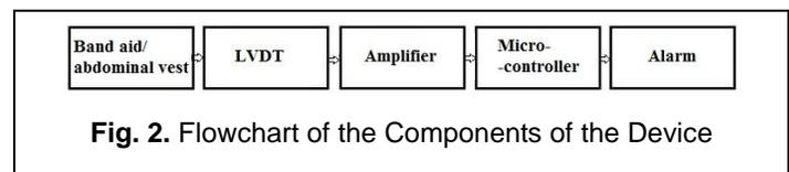
Fig. 2. Flowchart of the Components of the Device
