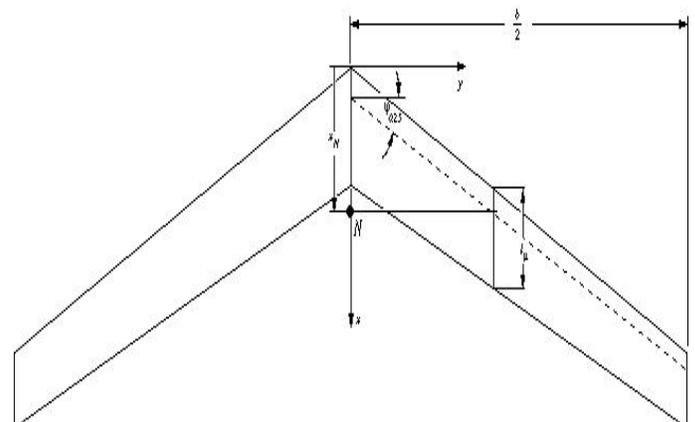
**Geometric parameters of a tapered, swept wing**
