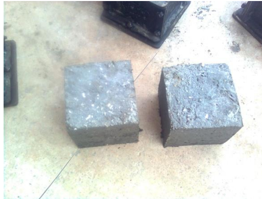
De-molding of IDRT Mix cubes after 24hours
