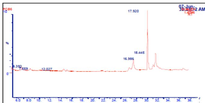
Figure 2.1 Chromatogram Standard - PCB Eluting at Retention Time 17.98 min
