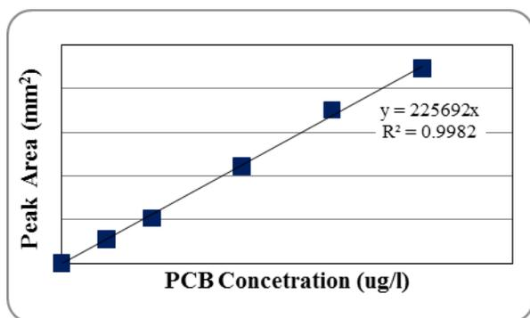
**Figure 2.4 PCB Standard Curve.**
