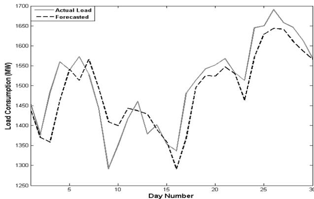
**Fig. 4.** Load forecasting results by the proposed hybrid method
