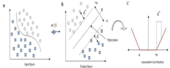
**Fig. 1.** The conceptual illustration of SVR model: a) data input in the original nonlinear input space, b) conversion to a linear problem in a higher dimension problem & 3)  $\epsilon$ -insensitive loss function
