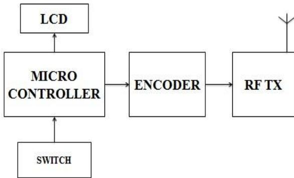
Fig. 1 Block diagram of Transmitter
