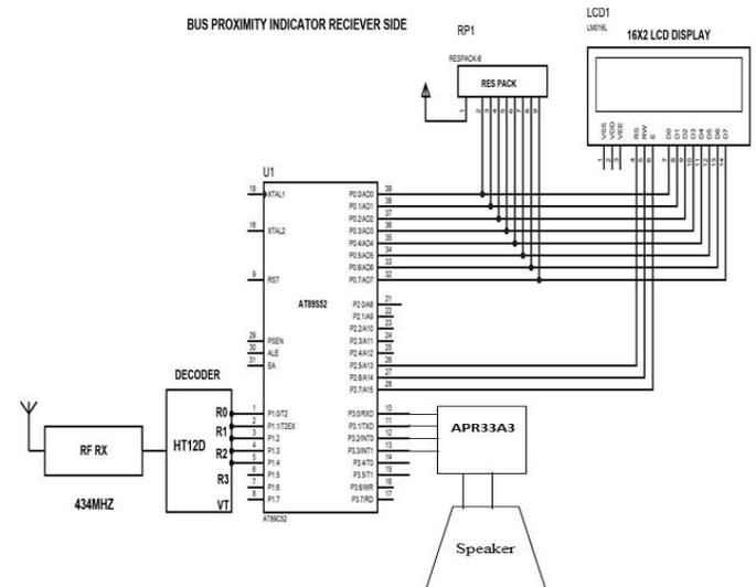
Fig.4 Receiver circuit diagram
