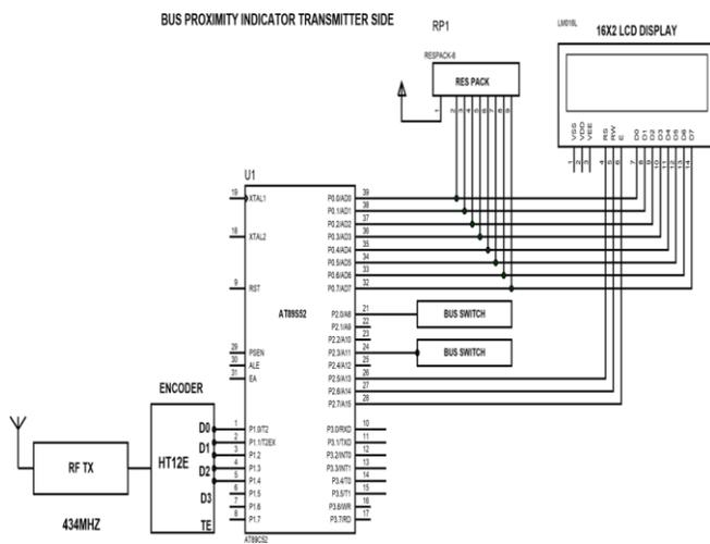
Fig.3 Transmitter circuit diagram
