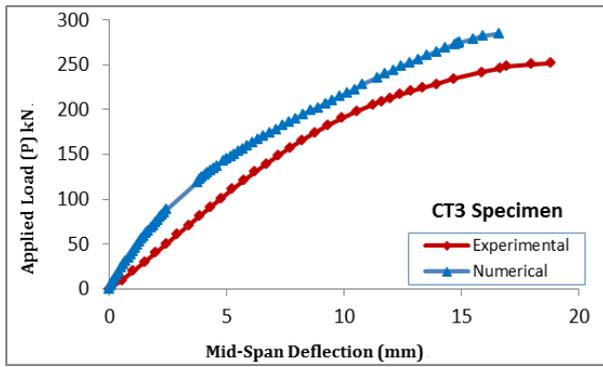
Figure (13) Numerical And Exp. Load-Deflection Curve
