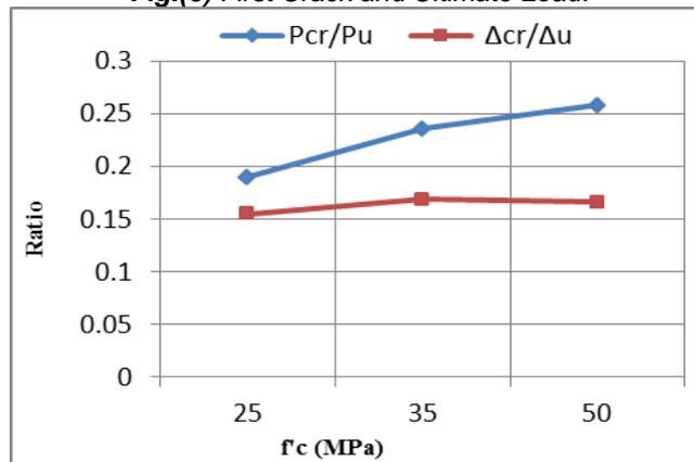
**Fig.(7)** Percent of First Crack Load to Ultimate Load with Deflection for Beams.
