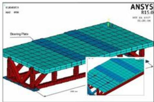
Fig. (10) Geometry of the Numerical Model.
