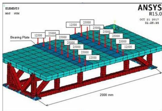
Figure (11) Distribution of Applied Load and Boundary Conditions
