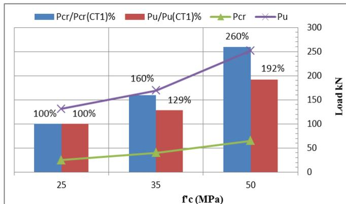
**Fig.(8)** ratio of first cracking and ultimate load of various compressive strengths in relation to the control beam.
