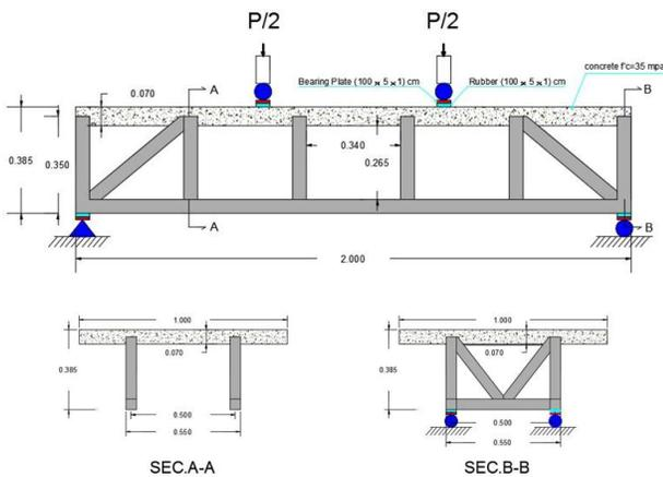
Fig.(1). Details Of Specimen (m)
