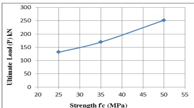
Fig. (5) Ultimate Load Various According To Concrete Compressive Strength.
