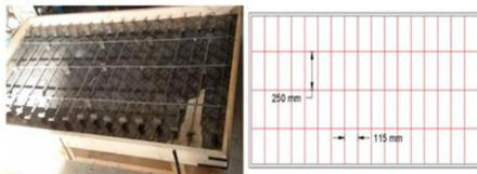
Fig.(2). Framework and Reinforcement Distribution
