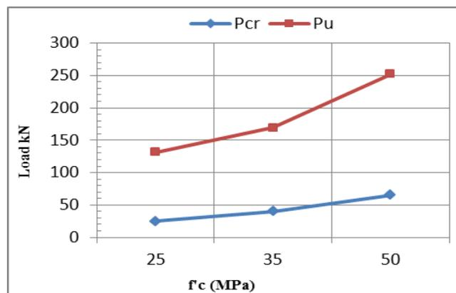
Fig.(6) First Crack and Ultimate Load.
