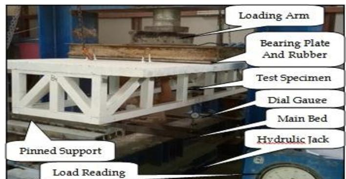
Fig. (3) Details of The Tested Machine.
