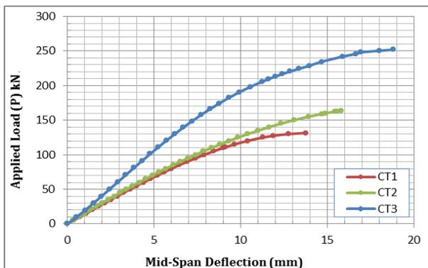
Fig. (4) Load –Deflection relationships for composite beams.
