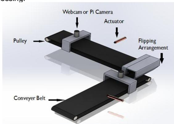
Fig: 4 proposed conveyor system
