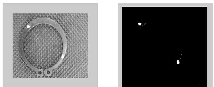
**Fig: 8** Defective Circlips
