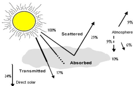
Fig. 3: percentage of solar energy that reach the surface.
