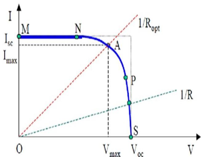
Figure 11: characteristics curve for PV cells [12].
