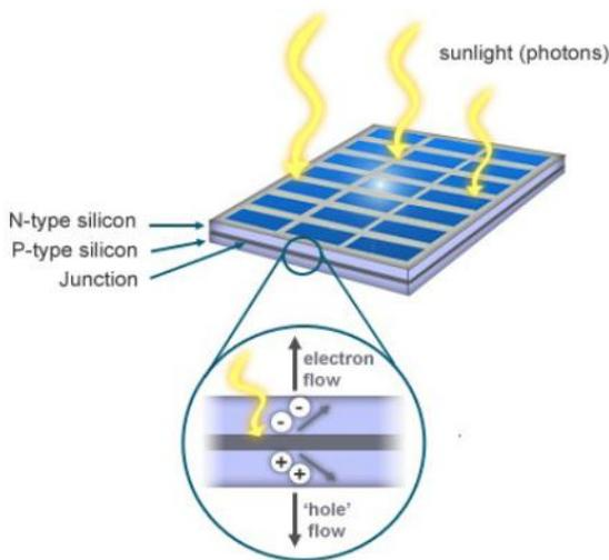
Fig 5: Photovoltaic effect.
