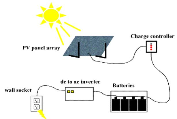
Figure 6: Components of a PV system.
