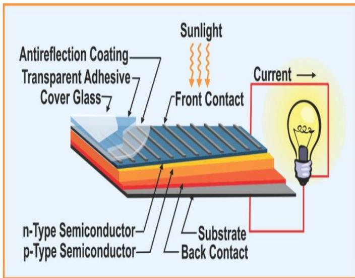
Figure 7: Basic Components of a c-Si PV Cell [3].
