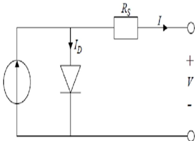
Figure 10: PV simple model [12].
