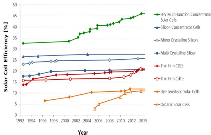
Figure 8: PV typical efficiencies [6].
