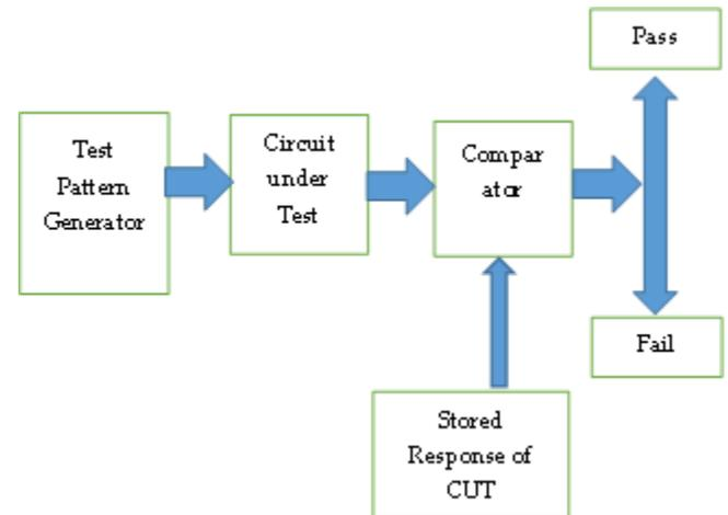
**Fig.1.** Testing of CUT
