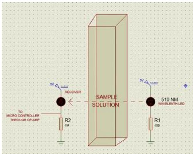
Fig.2. Transmitter and Receiver Section
