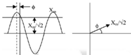
**Figure 3: Phasor representation of sinusoidal signal**
