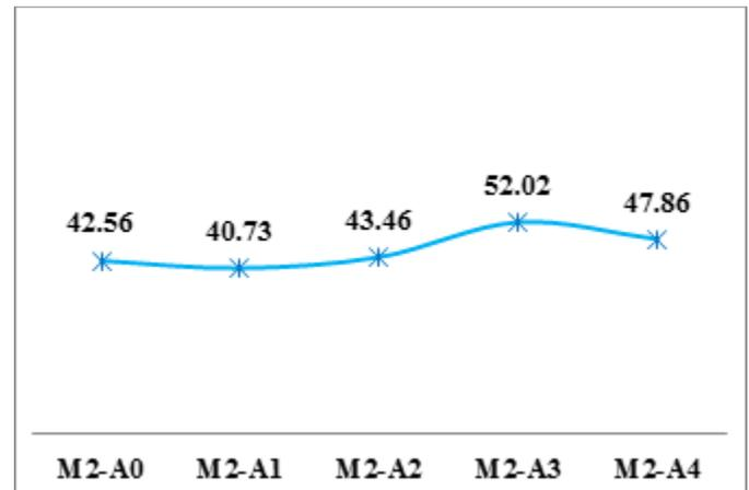
Fig.3.Ultimate capacity of M30 grade tubular column
