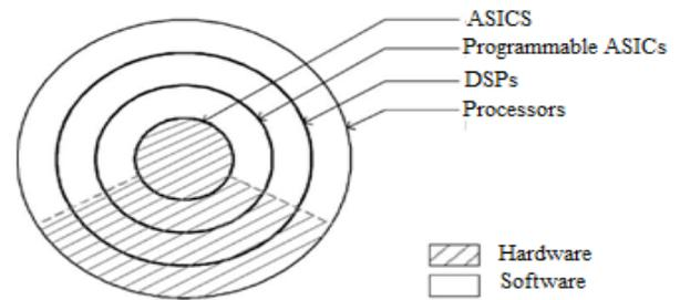
Fig 2. Various Implementation Approaches And Hardware–Software Relationship
