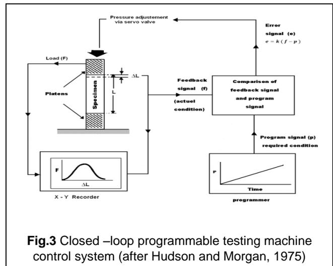
Fig.3 Closed –loop programmable testing machine control system (after Hudson and Morgan, 1975)
