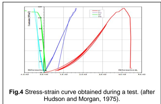
Fig.4 Stress-strain curve obtained during a test. (after Hudson and Morgan, 1975).
