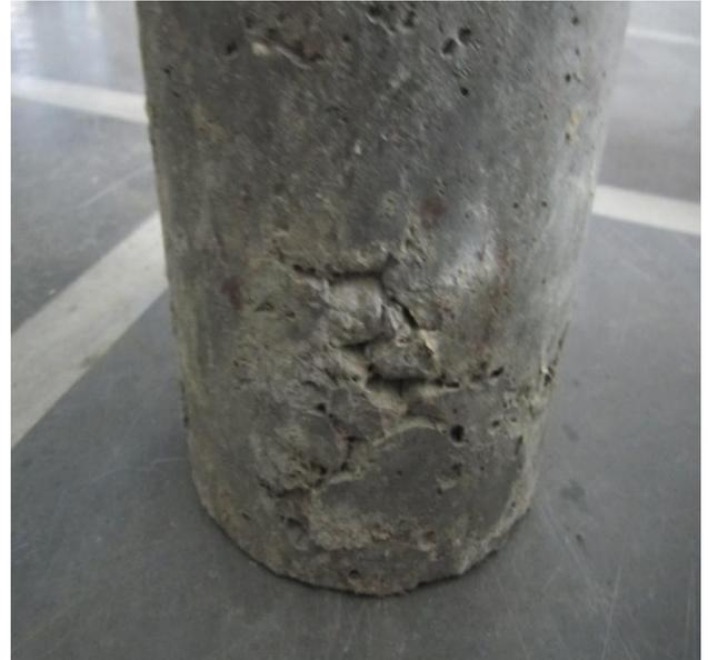
**Fig 10:** Voids in cylinder for 1.5% fiber-cement ratio though properly compacted
