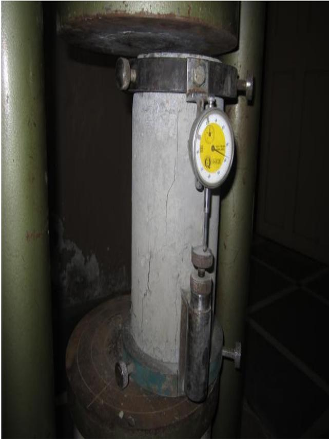
Fig 1: dial gauge set up to obtain stress-strain deformations
