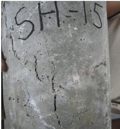
**Fig 9:** Cylinder resistance to cracking due to fibers
