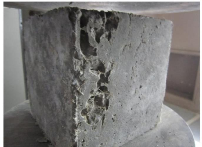
**Fig 11:** Voids in cube for 1.5% fiber-cement ratio though properly compacted
