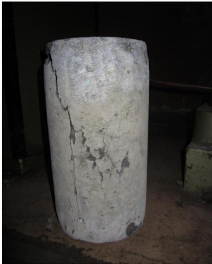
**Fig 7:** bulging in concrete with fibers
