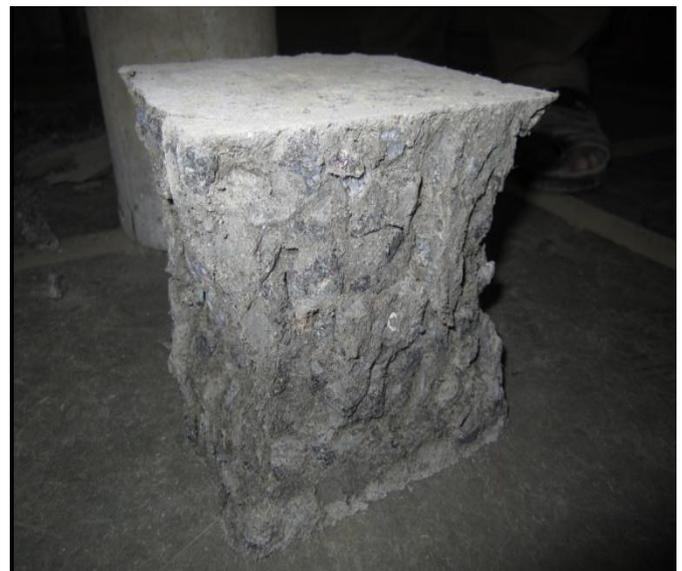
Fig 6: cube failure pattern in M30 plain concrete
