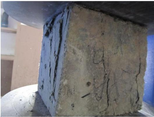
**Fig 8:** Cube resistance to cracking due to binding of fibers
