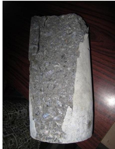
Fig 5: cylinder failure in M30 plain concrete
