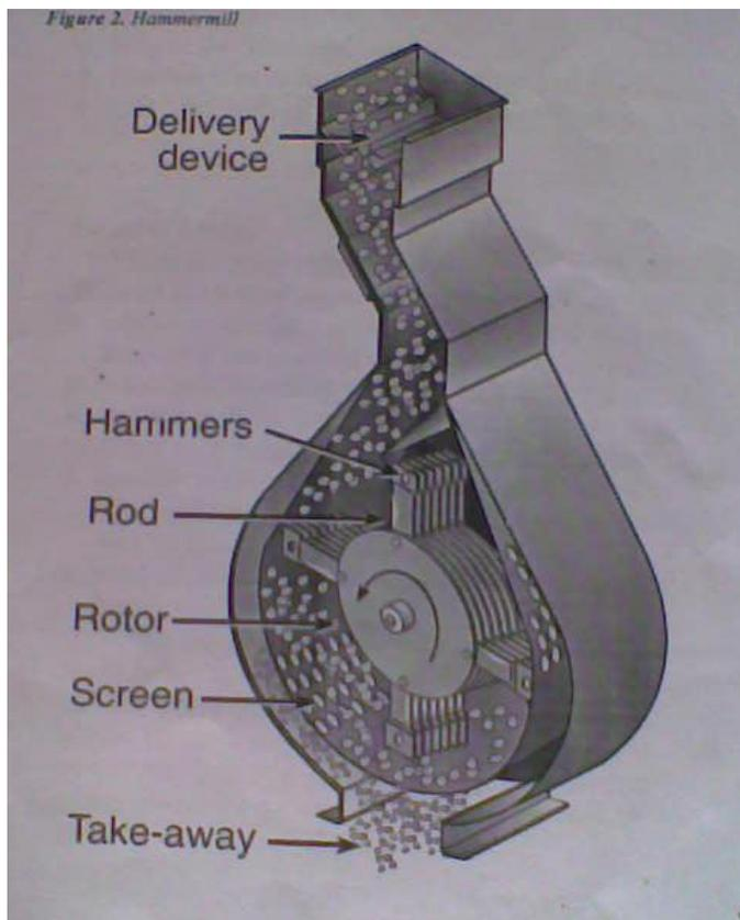
**Fig.1** Main Components of Hammer Mill [2]
