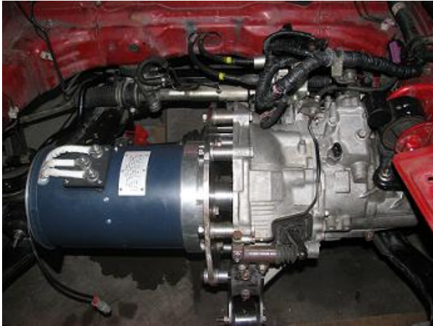
Figure 2: 3 Phase Induction Motor
