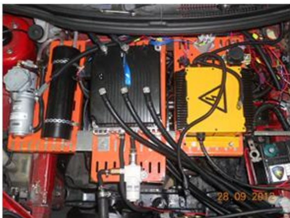
Figure 8: Electrical System layout
