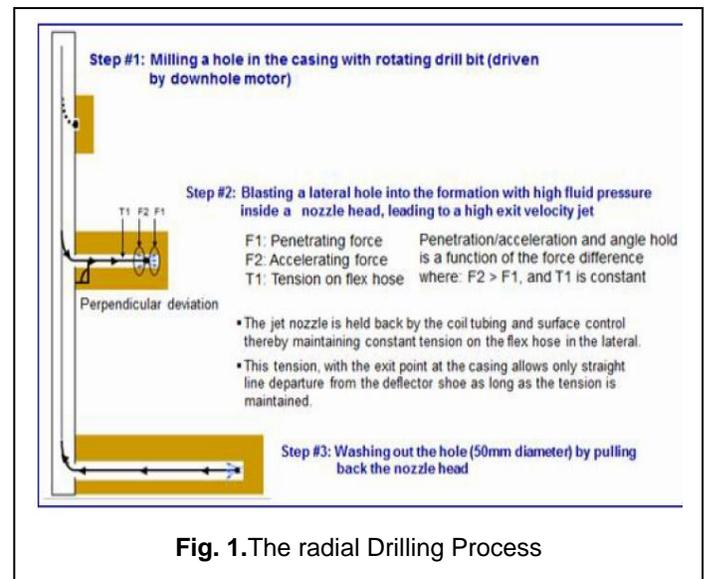
This will help reduce the number of work-over jobs perfield/reservoir. After radial drilling is done the filed can be produced for other one-two years without much of workover/IOE-EOR jobs mostly. After that work-over jobs can be taken up to stimulate the previously damage zone as well as zone extracted through radial drilling techniques.
