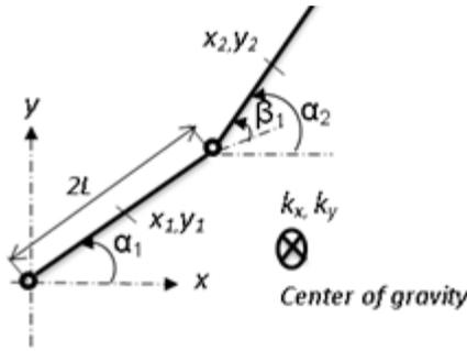
Figure 2: The module angle of the planar snake robot
