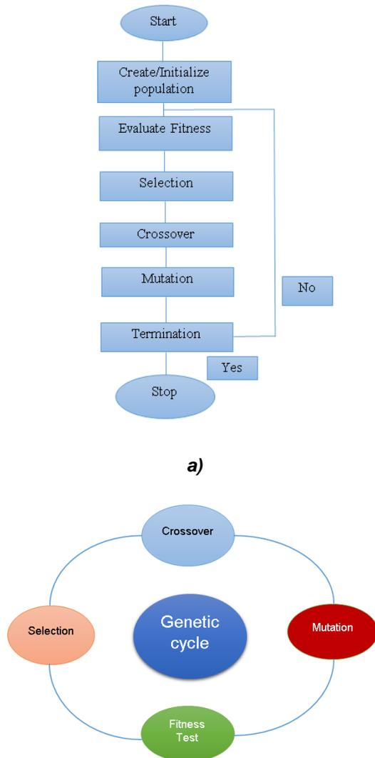
**Figure 12:** a) Flow diagram of genetic algorithm b) Genetic cycle
