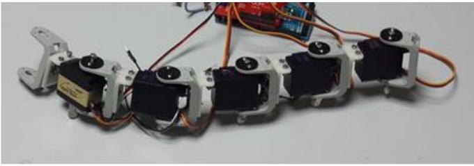
Figure 1: Photograph of the snake robot TAROBOT-1
