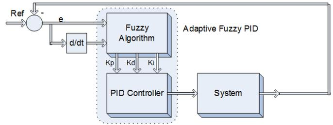
Figure 6: The block structure of the control system and a fuzzy controller
