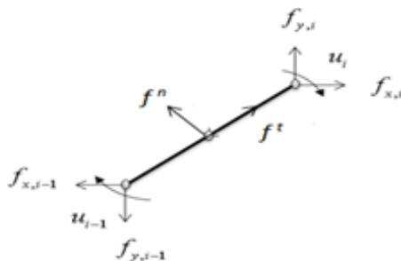
**Figure 4:** The forces and moments acting on each module of the snake robot
