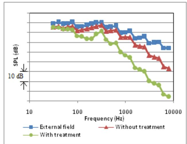
Fig. 6. Inner acoustic fields of cylinder with and without NCT
