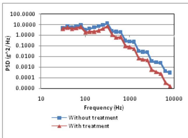
**Fig. 7.** Vibration response of cylinder with and without NCT
