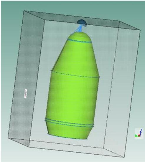
Fig. 4. PLF modeled within the chamber
