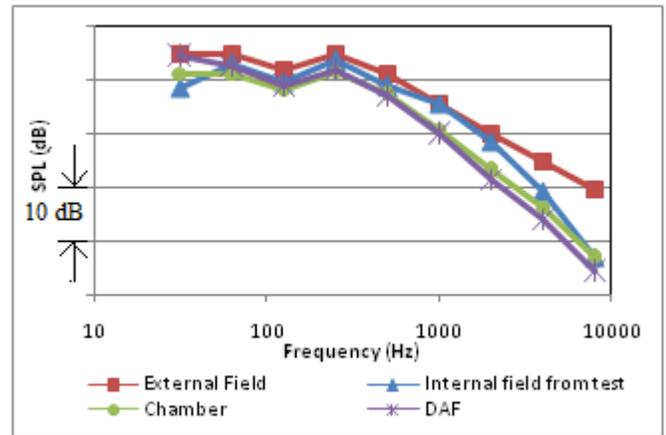
Fig. 5. Comparison of inner acoustic field of cylinder with excitation modeled as chamber (energy constraint) and DAF with that obtained from test
