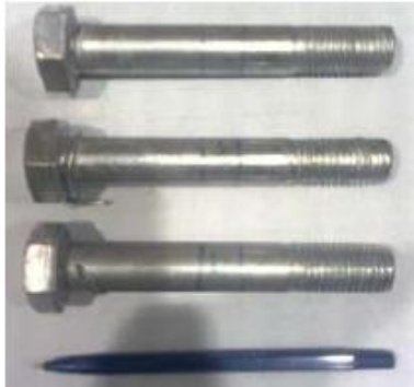
Figure 1. Sample testing results bolt A325 Hot Dip Galvanized
