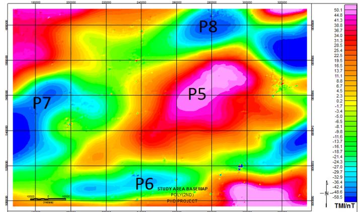
**Fig. 2 (b)** Residual TMI base map of the study area indicating the modeled points [14].
