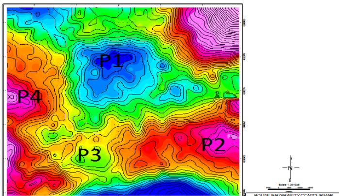
**Fig. 2 (a)** Residual Bouguer gravity base map of the study area indicating modeled points [14].
