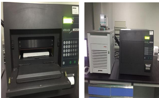
Fig. 7 (A) Left: Heat flow meter (Netzsch HFM 436) (Closed) with prepared VIP (B) Right: Heat flow meter (Netzsch HFM 436) (Opened) with prepared VIP sample
