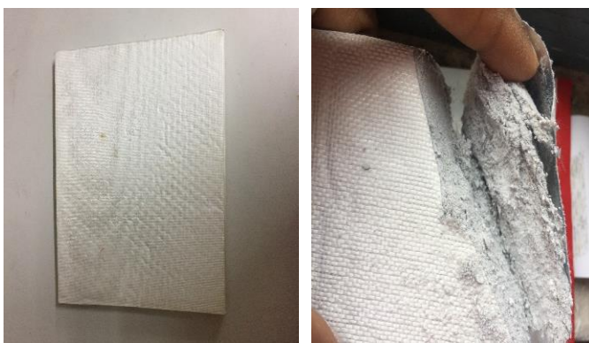
Fig 4: (a) VIP with hybrid core material of fly ash, fumed silica and glass fiber (b) Cut section of the VIP showing its core material
