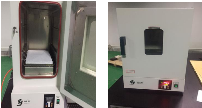
Fig 6: (A) Left: High temperature furnace (Open) with prepared VIP (B) Right: High temperature furnace (Closed) with prepared VIP.
