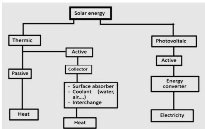
Fig. 1. Synoptic scheme of the direct use of the solar energy
