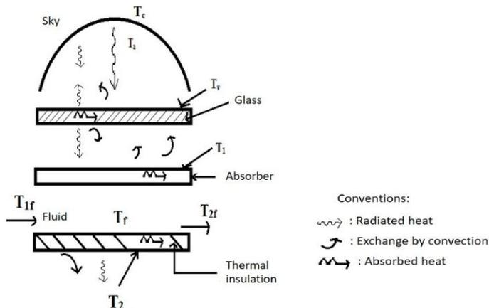
Fig.3. Operating principle of a solar collector
