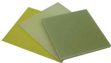
Fig. 3. FR-4 sheet used for antenna fitting
