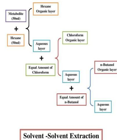
**Figure 03:** Solvent extraction by compatible solvents
